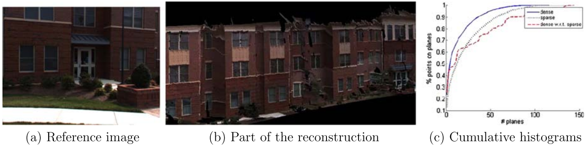
Fig. 11 (Color online) Evaluation of the use of priors. The dotted black curve is the cumulative histogram of the sparse points for the image of a . The x-axis for the dotted black curve refers to the planes sorted in descending order with respect to the number of points they contain. The solid blue curve is a similar histogram for the dense re-
