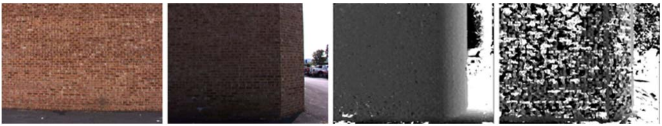
Fig. 10 (Color online) Left : two video frames, middle : gain corrected stereo, right : standard stereo
