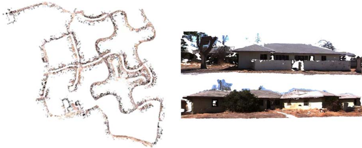
Fig. 1 (Color online) View from above and details of reconstructed models from a 170,000 frame video
