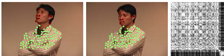
Fig. 3. ( left and middle ) A sequence of a person moving with his head rotating around the neck. The color of a dot, red or green, shows the segmentation result. There is one misclassification, the red dot on the left shoulder. The other red dot on the left arm is an outlier. ( right ) The affinity matrix of locally estimated subspaces is shown. The row and columns are rearranged based on the segmentation.
