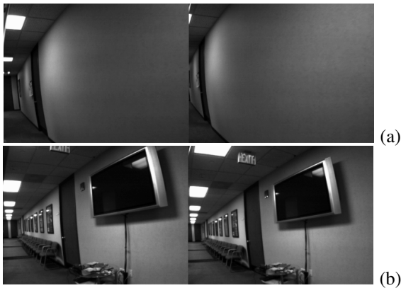
Fig. 6. Matching examples from the two loops of the Corridor sequence. Matching works well even for quite featureless images (a).
